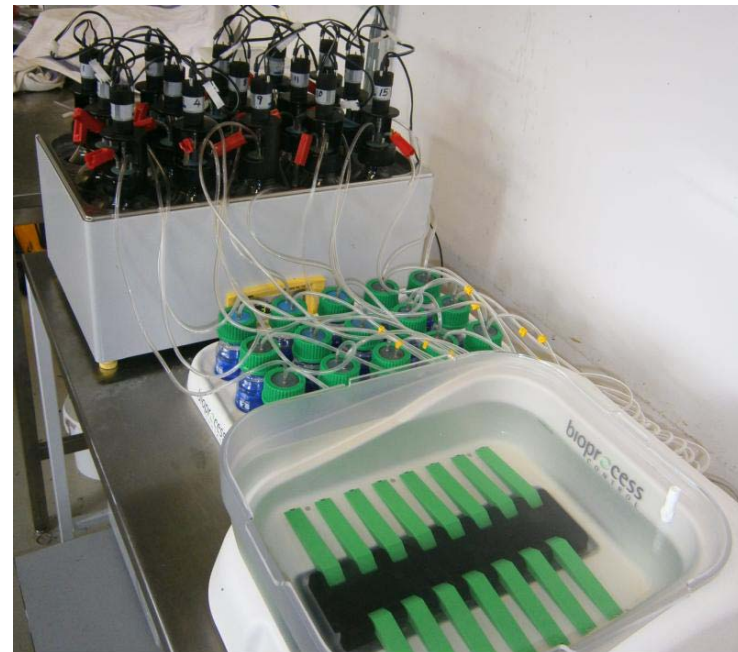
Bioprocess BMP unit used to obtain specific methane yield
